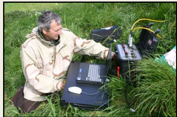
Fig 12. Paul Cheetham operating the Electrical Resistance Tomography (ERT) meter at Clandon Barrow in 2009.
