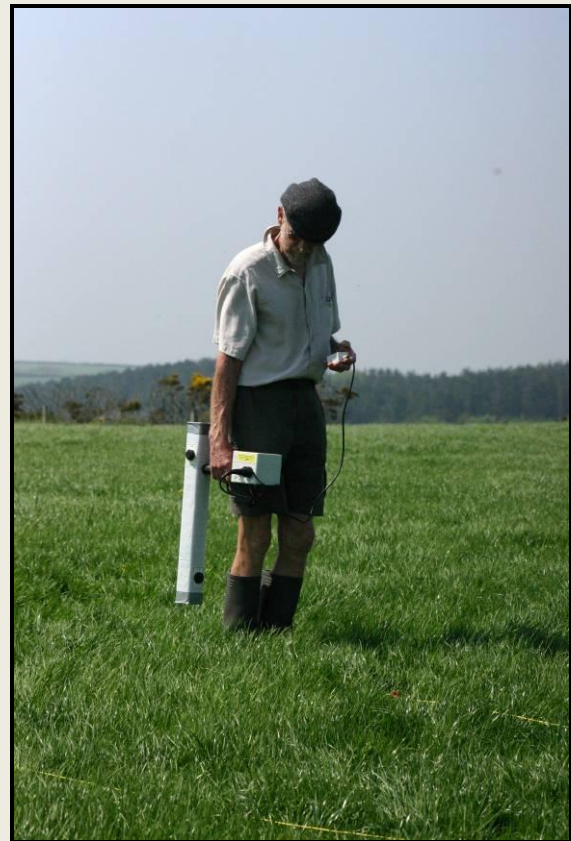
Fig 2. A Volunteer undertaking geophysical survey at Bronkham Hill in 2008 using a Geoscan FM36 Fluxgate Gradiometer
